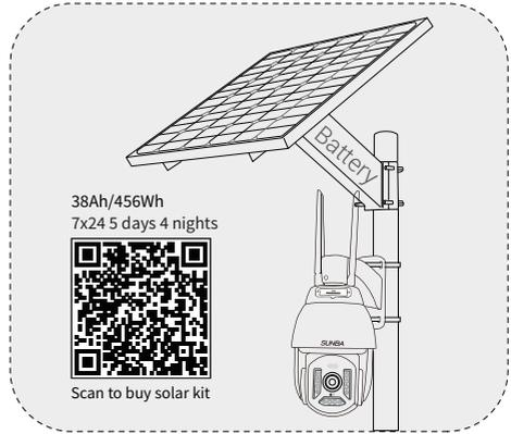
Warning: The load end for MANY battery charge controllers doesn't regulate voltages and is for wide voltage equipments. Sunba cameras require, however, fixed voltage. In this case, you need to get a voltage regulator for the load end if the battery doesn't have built-in regulators.
